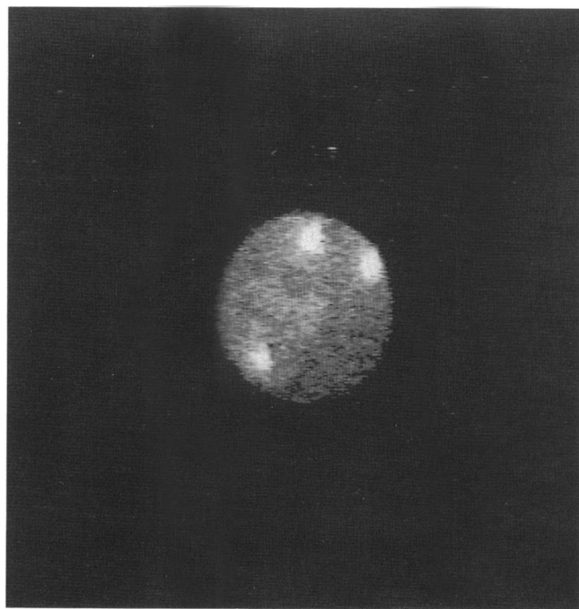
FIGURE 2 Fluorescent microspheres 1 \mu\text{m} in diameter as seen through a diaphragm 10 \mu\text{m} in diameter.
